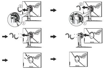
• Use only the UL Listed Wall Mount Bracket with minimum weight/load 28.8 kg (Screw size: M4 x 10 mm).
