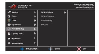
By activating this function, this monitor displays two pictures, three pictures or four pictures for any video source.
