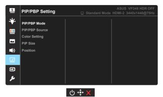
By activating this function, this monitor displays two pictures from one or two video sources.
