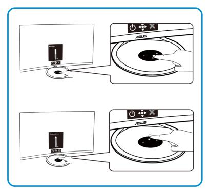
There is convenient control key for the speaker volume and Halo Lighting brightness on the transparent base.
