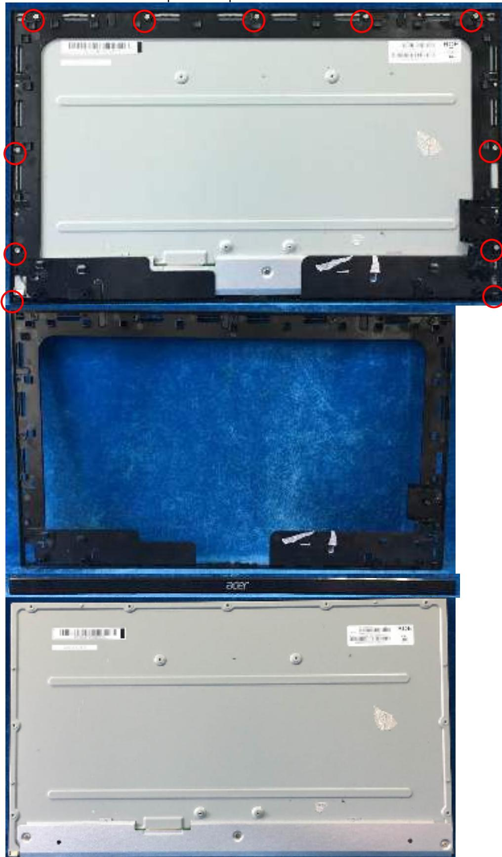
S6 Firstly, unscrew the screws of the main board and pull out the two screw bolt to remove the mylar. Then unscrew the screws of the power board and main board to remove them from mainframe.
